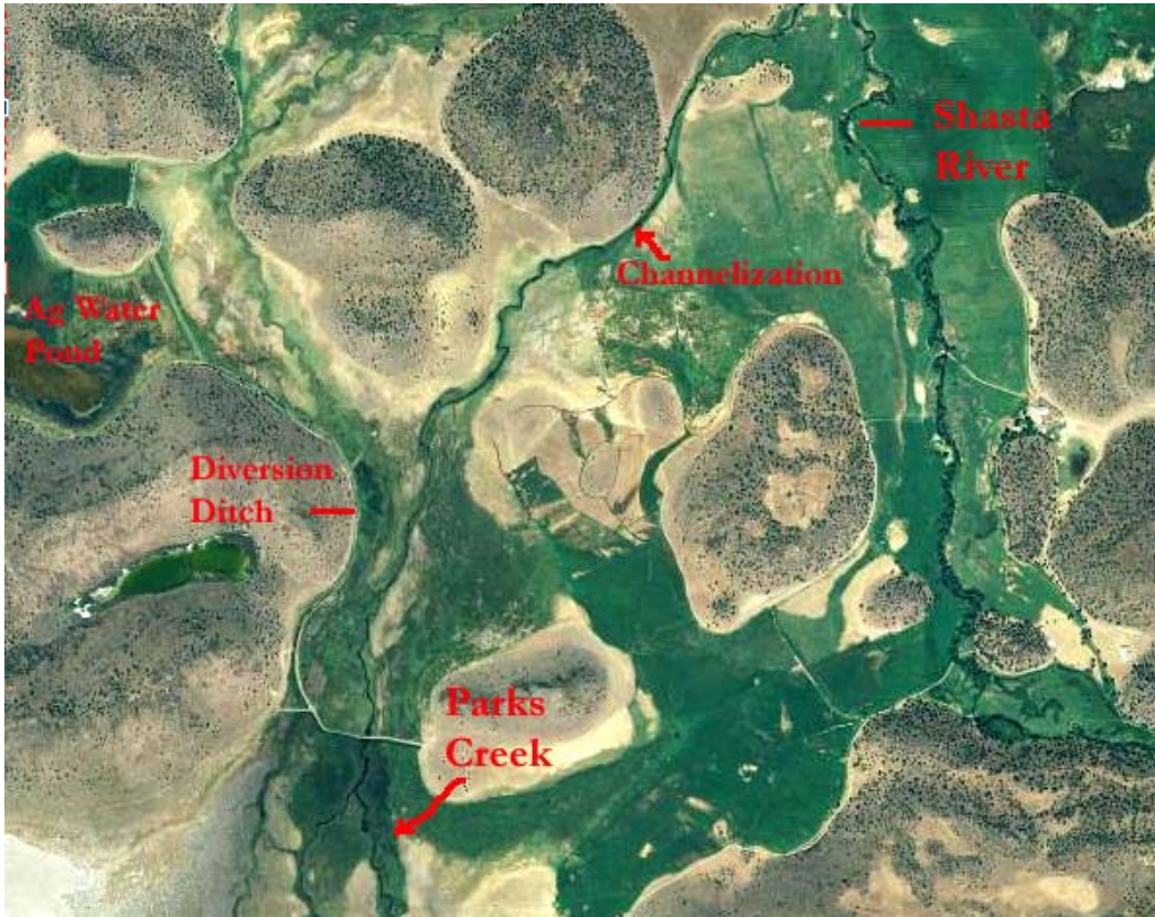
Figure 4. Lower Parks Creek is shown here in a 2005 aerial photo that demonstrates dewatering, channelization and loss of fisheries productivity in what could easily be converted into a refugia.
