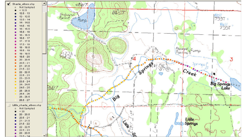
Figure 39. Thermal infrared radar (TIR) map of Big Springs Creek shows that the stream warms rapidly as a result of diversion and now is too warm for optimal salmonid rearing within a distance of less than three miles. Data from Watershed Sciences (2003) provided as GIS by NCRWQCB staff.
