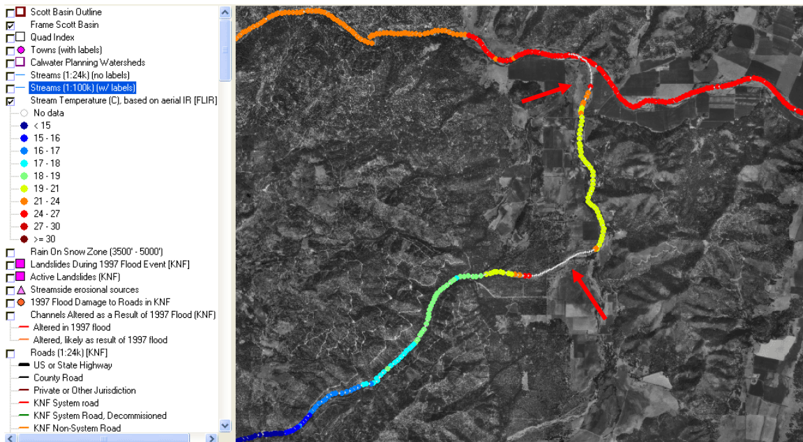
Figure 7. This map shows summary data of Scott River Thermal Infrared Radar (TIR) surveys for Shackleford Creek. Note that water temperature warms in a downstream direction as flow is depleted. Reaches with no temperature coded color are dry (red arrows). Data from Watershed Sciences (2004).
