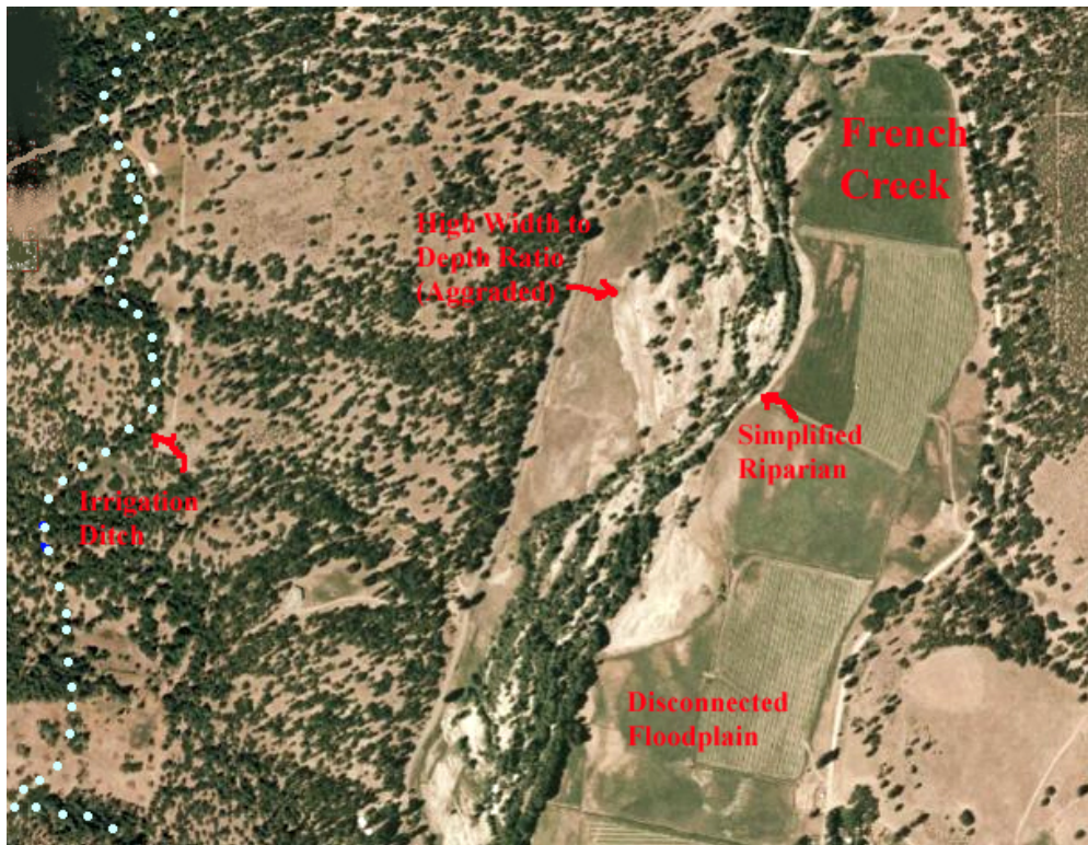
Figure 10. French Creek in an alluvial valley reach, which would have been optimal for coho historically, shows degraded riparian conditions, signs of sediment over-supply, flow depletion and disconnection from the floodplain. Aerial photo 2005.
