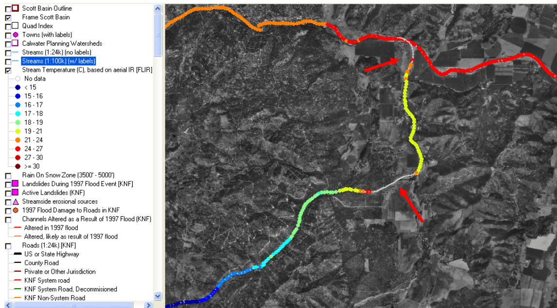
Figure 7. This map shows summary data of Scott River Thermal Infrared Radar (TIR) surveys for Shackleford Creek. Note that water temperature warms in a downstream direction as flow is
