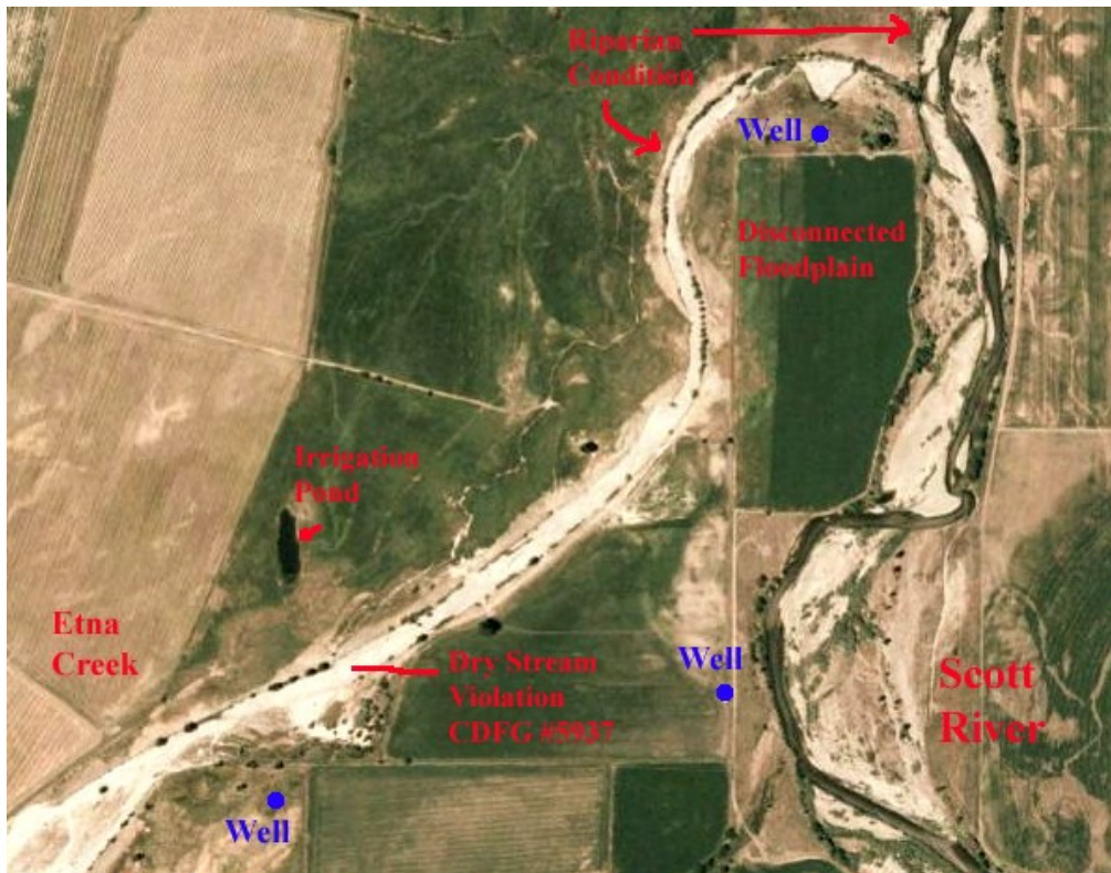
Figure 8. The mainstem Scott River and Etna Creek are confined, channelized and disconnected from wetlands and springs that likely provided coho salmon refugia before human disturbance. Note also that wells next to streams have the potential to deplete cold subsurface contributions. Aerial photo from is from 2005.
